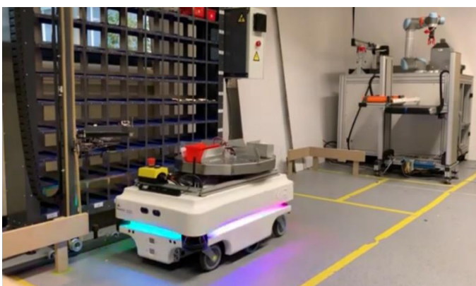
Fig. 3. An automated ground vehicle that aims to make the production environment autonomous by transporting products between two given points ( www.fontys.nl/robotica ).
