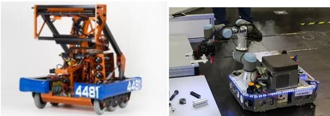
Fig. 2. Two educational mobile robot, designed for the RoboCup competition to carry different object with various shapes throughout unstructured environments at Fontys University of Applied Sciences ( www.fontys.nl/robotica )
