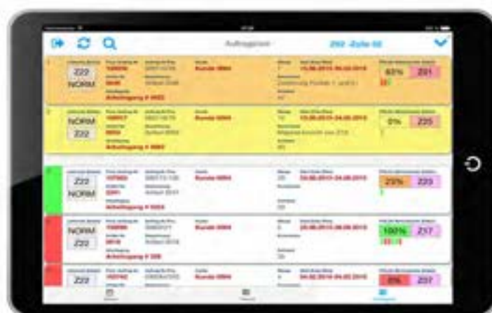
Example of the Timeaxx digital POLCA screen. Availability of cards is displayed by a percentage on the right side of the screen. (Source: axxelia).
