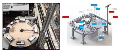
system checks the parts on the index table. When a product is approved, it is pushed off the index table by a cylinder. The product then ends up on the discharge conveyor.
